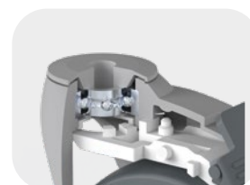
Section Picture: Swivel Head with Ball Bearing 6203 2RS DIN 625
